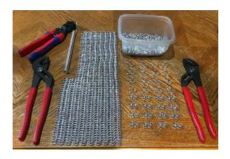
The small coil of wire on the left is ready to be cut into rings. On the right are several small "fivelet" units ready to be added to complete the row, and several rings ready to join them with.
